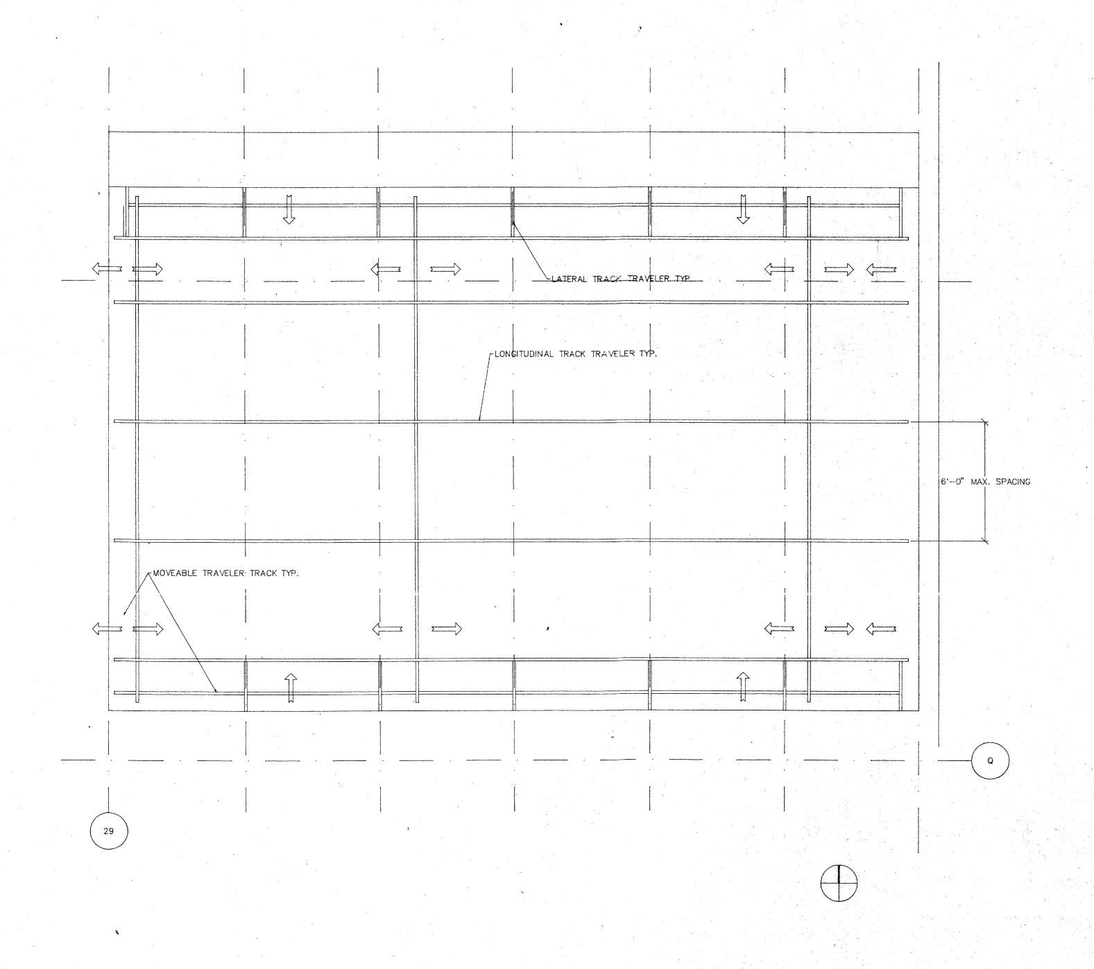
REFLECTED CEILING PLAN SHOWING TRAVELLER TRACK SCALE: 1/4"=1'-0"
