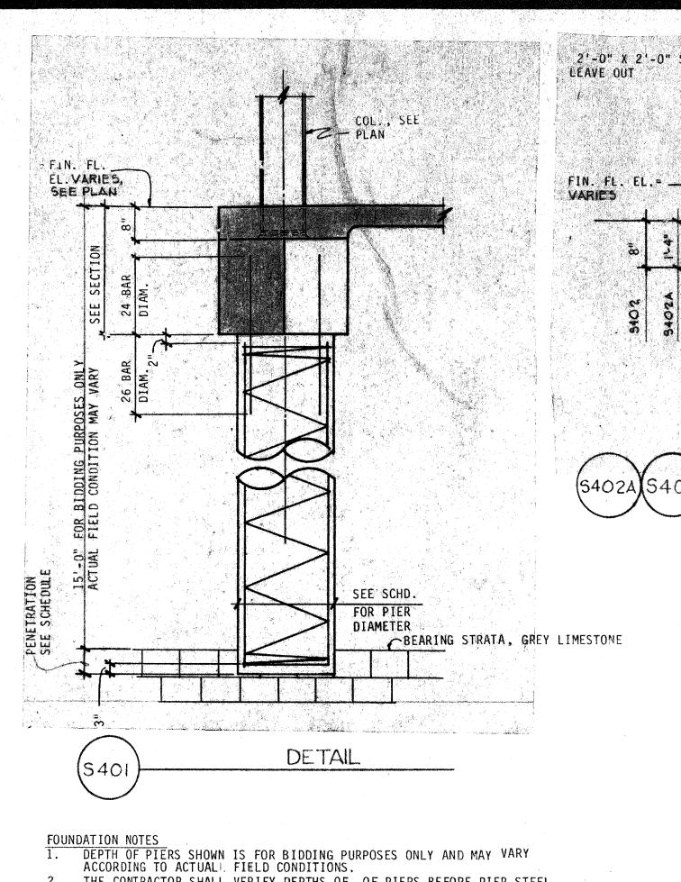
THE CONTRACTOR SHALL VERIFY DEPTHS OF OF PIERS BEFORE PIER STEEL IS CUT. PIER STEEL SHALL BE DELIVERED TO THE JOB SITE IN STOCK LENGTHS AND CUT AS REQUIRED.
