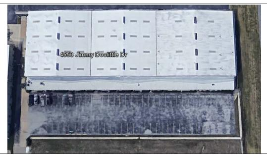
**Violation 1 -** There are no accessible parking spaces provided where three (3) are required, one of which is required to be van accessible
