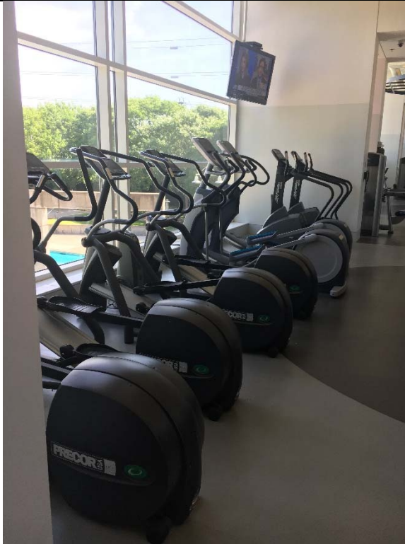
Violation 55 - Not all of the exercise equipment has the required clear floor space provided next to it.
