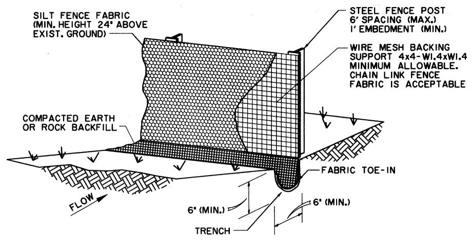
SILT FENCE SHOULD BE SECURELY FASTENED TO BACKING SUPPORT AND POSTS.
