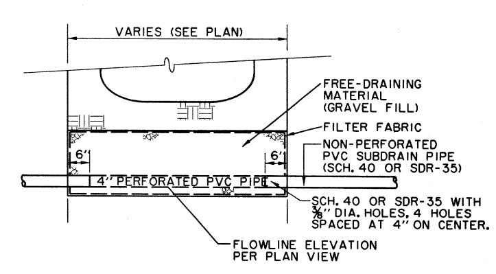
SUBSURFACE DRAIN SYSTEM DETAIL (SECTION PARALLEL TO CURB)
