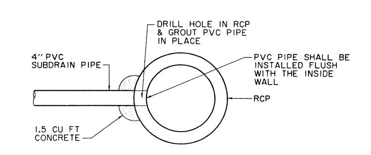
PVC SUBDRAIN PIPE CONNECTION TO STORM DRAINAGE PIPE N.T.S.
