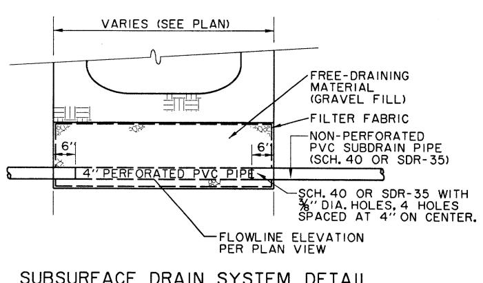
SUBSURFACE DRAIN SYSTEM DETAIL (SECTION PARALLEL TO CURB) N.T.S.
