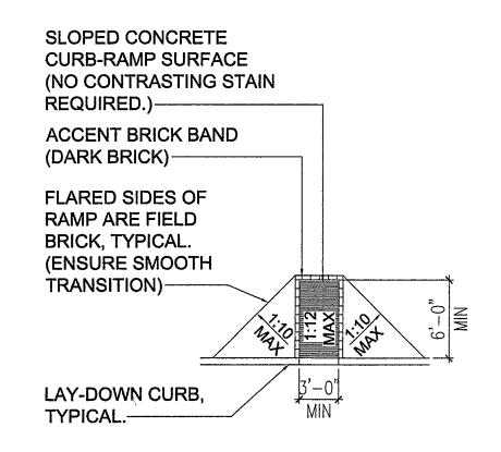
NOTE: SLOPED CONCRETE CURB-RAMP SURFACE TO HAVE FORMED OR SAWCUT GROOVES 3/4" WIDE X 1/4" DEEP @ 2" ON-CENTER, FORMED PERPENDICULAR TO THE PATH OF TRAVEL, TYPICAL.
