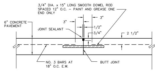
NOTE: CONSTRUCTION JOINT SHOULD BE FORMED WHENEVER THE PLACEMENT OF CONCRETE IS SUSPENDED FOR 30 MINUTES OR MORE.
