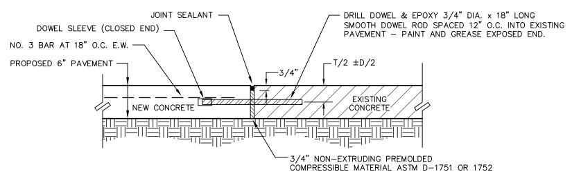
NEW CONCRETE TO EXISTING CONCRETE DETAIL (TO BE USED ON ALL TAXI-WAY PAVING) NOT TO SCALE
