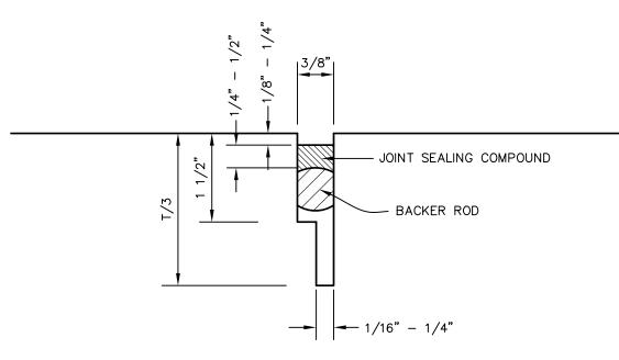
NOTE: T = PAVEMENT THICKNESS.
