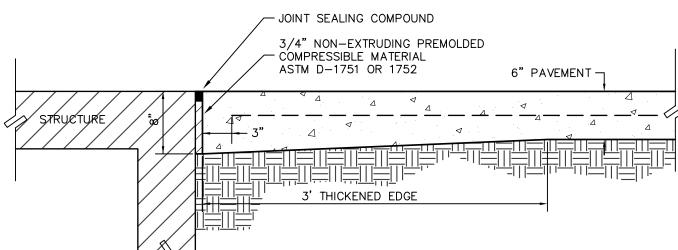
EXPANSION JOINT AT STRUCTURE DETAIL NOT TO SCALE
