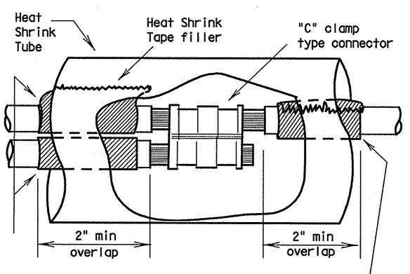
Seal between Conductors with heat shrink tape. Tape to extend past end of tubing by 1/8 " to 1/4 ".
