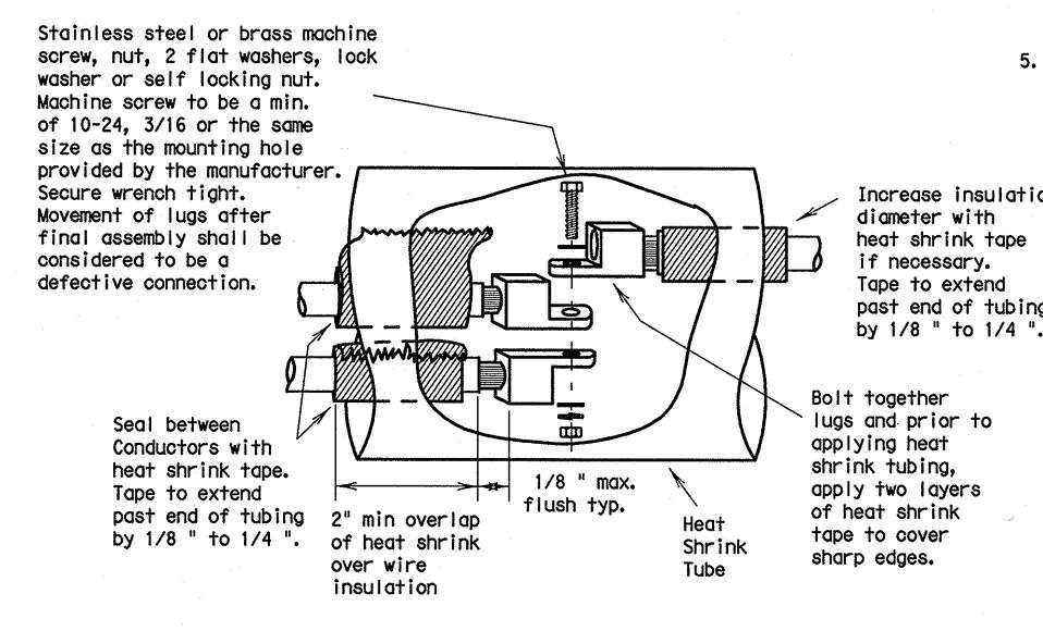
SPLICE OPTION 2 BOLTED WIRE LUGS SPLICE OPTION 3 SPLIT BOLT
