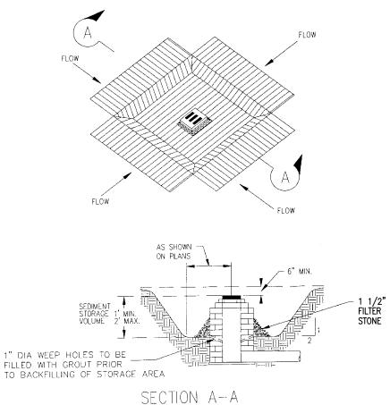
EXCAVATED DROP INLET PROTECTION
