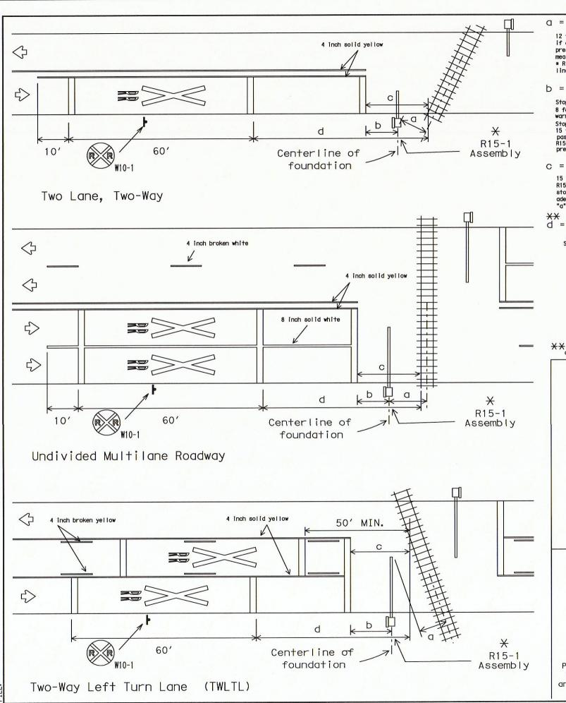
12 feet minimum, 15 feet usual, if active warning devices are present. Distance "a" should be measured from the centerline of \* R15-1 assembly to the centerline of nearest track.
