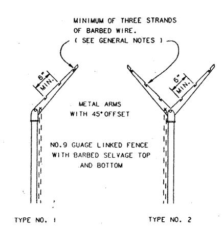
FENCE POST SHALL BE SET BACK SO BARBED WIRE DOES NOT EXTEND OVER PROPERTY LINES. TYPE NO. I ARMS SHALL BE INSTALLED ON SIDE AWAY FROM AIRPORT PROPERTY OR AIRCRAFT OPERATIONS AREA.
