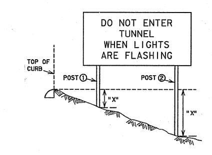
The "X" dimension is the elevation difference at the post between the ground and the edge of pavement or top of curb.
