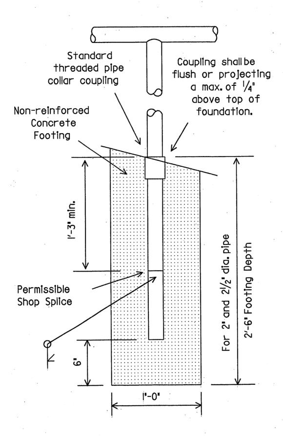
Pipe collar coupling shall be used for all signs supported on 2" and 2 1/2 " diameter pipe post.
