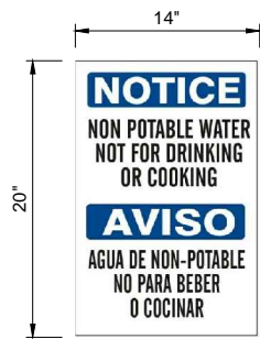
4 E-201 NON-POTABLE WATER SIGN SCALE: NONE NOTES: 1. SIGN SHALL BE INSTALLED ON A SQUARE BREAKAWAY SIGN SUPPORT. SEE SPECIFICATIONS FOR DETAILS. 2. BOTTOM OF SIGN SHALL BE INSTALLED FIVE FEET FROM EXISTING GROUND.
