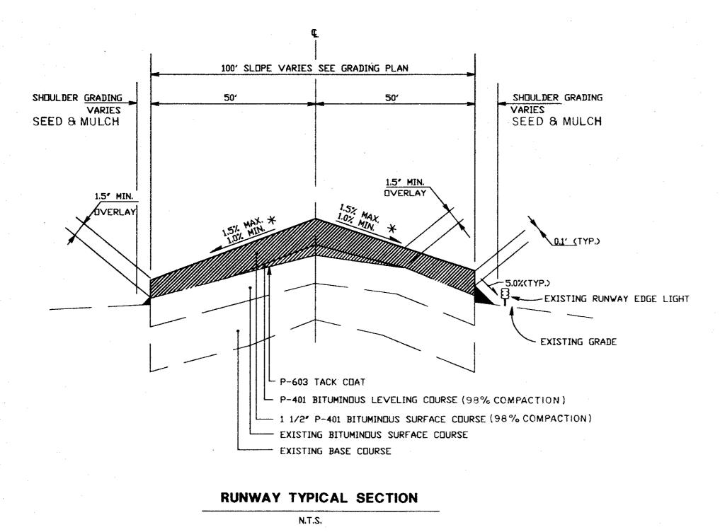
\* 1.0 % MINIMUM SLOPE ALONG RUNWAY, EXCEPT AT TAXIWAY INTERSECTIONS FOR TAXIWAY'S A,C AND F. SEE TAXIWAY PROFILE SHEETS 9 AND 10, AND PAVING PLAN SHEETS 6-8.
