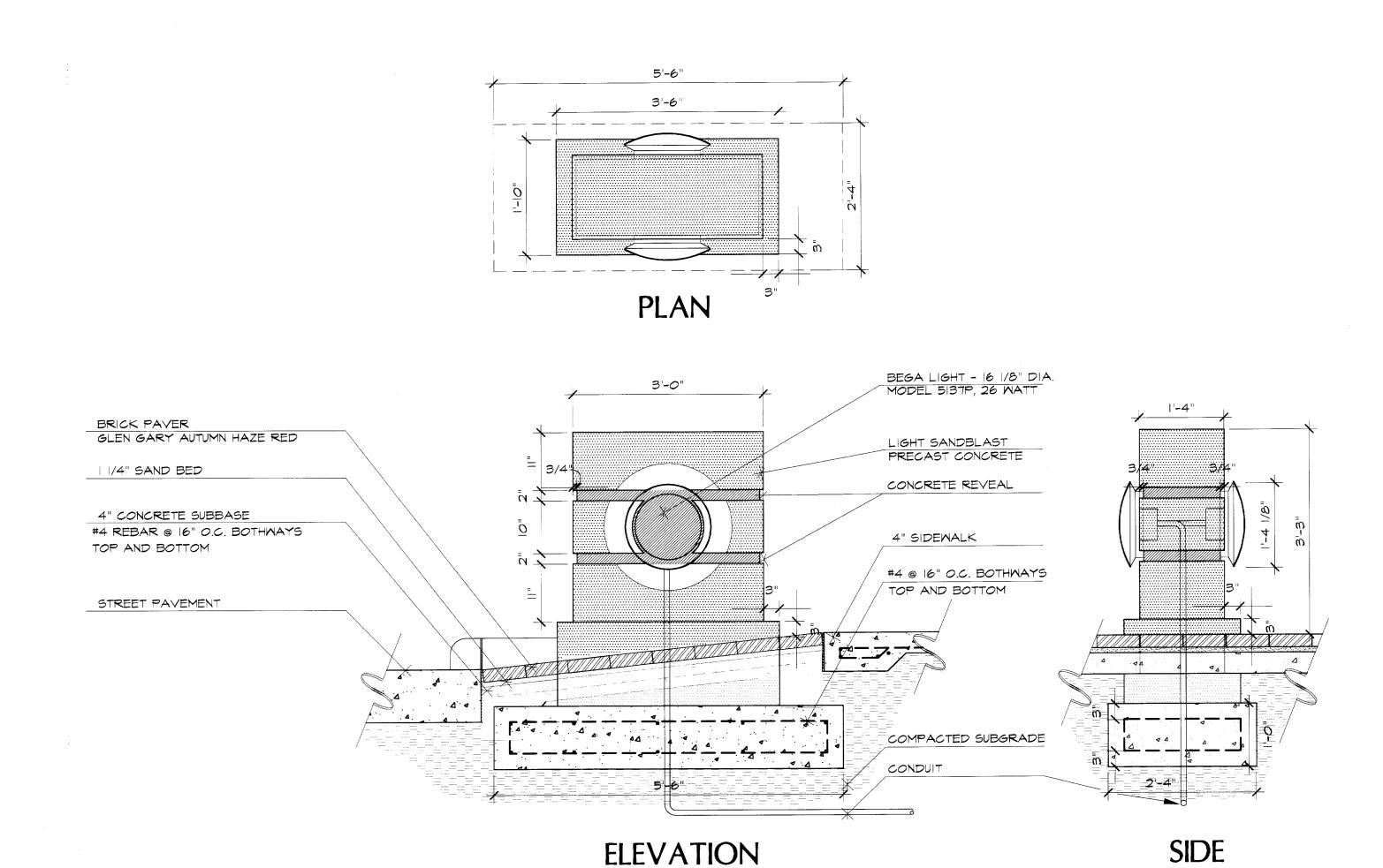
B CUSTOM PRE-CAST CONCRETE BOLLARD
