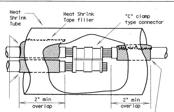
Seal between Conductors with heat shrink tape. Tape to extend past end of tubing by 1/8 " to 1/4 ".
