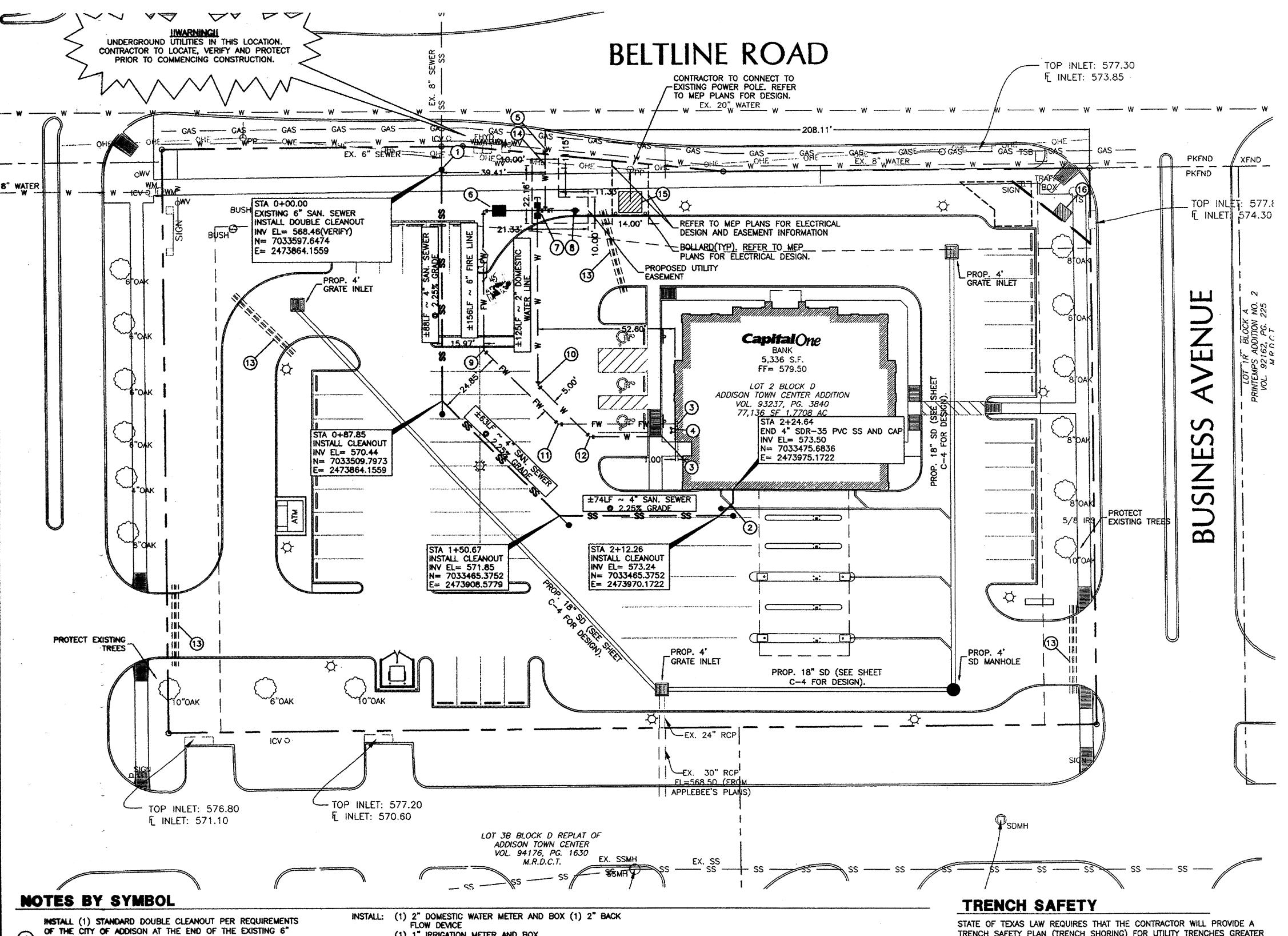
SANITARY SEWER PIPE. BEGIN 4" SDR-35 PVC SANITARY SEWER SERVICE LINE. CONTRACTOR TO VERIFY EXISTING INVERT AND LOCATION PRIOR TO INSTALLATION.
