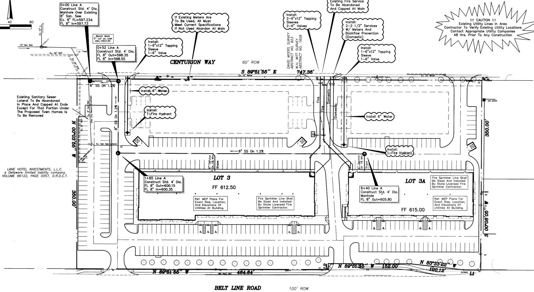
Existing Sanitary Sewer Lateral To Be Abandoned In Place And Capped At Ends Except For That Portion Under The Proposed Town Homes Is To Be Removed
