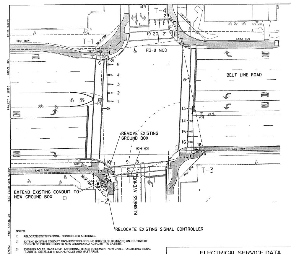
SPLICING OF SIGNAL CABLE, VIVDS CABLE, AND ELECTRICAL CABLE IS NOT PERMITTED. INSTALL NEW CABLE TO ALL EXISTING POLES AND EQUIPMENT.
