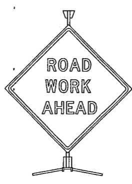
WOOD POST SIGN SUPPORT: for 48" x 48" warning sign.
