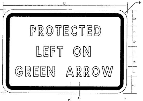
R10-12 24"x 30" LEGEND BLACK(NON-REFLECTIVE) BACKGROUND WHITE(REFLECTIVE) CIRCULAR GREEN(REFLECTIVE)
