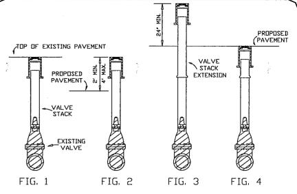
NOTE: The valve cover must always be exposed so the valve can be operated at any time. Exceptions must be approved by the engineer in advance.
