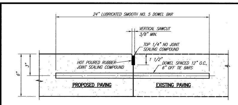
DOWEL BARS SHALL BE DRILLED INTO PAVEMENT HORIZONTALLY BY USE OF A MECHANICAL RIG. DRILLING BY HAND IS NOT ACCEPTABLE. PUSHING DOWEL BARS INTO GREEN CONCRETE IS NOT ACCEPTABLE.
