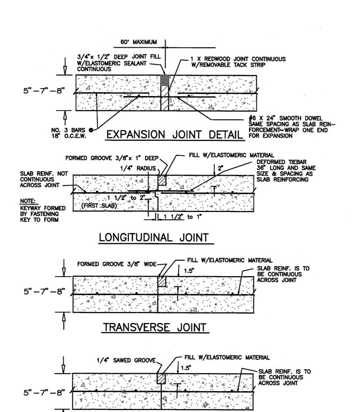
PAVEMENT JOINT DETAILS -NO SCALE-
