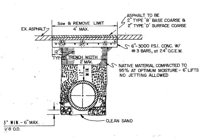
J TYPICAL BACKFILL WATER MAIN
