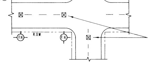
A BLUE STIMSONITE FIRE-LITE REFLECTOR (OR APPROVED EQUAL) TO BE PLACED IN THE CENTER OF STREET OPPOSITE FIRE HYDRANTS. THE INSTALLATION OF THIS REFLECTOR SHALL BE AS PRESCRIBED BY THE MANUFACTURER.
