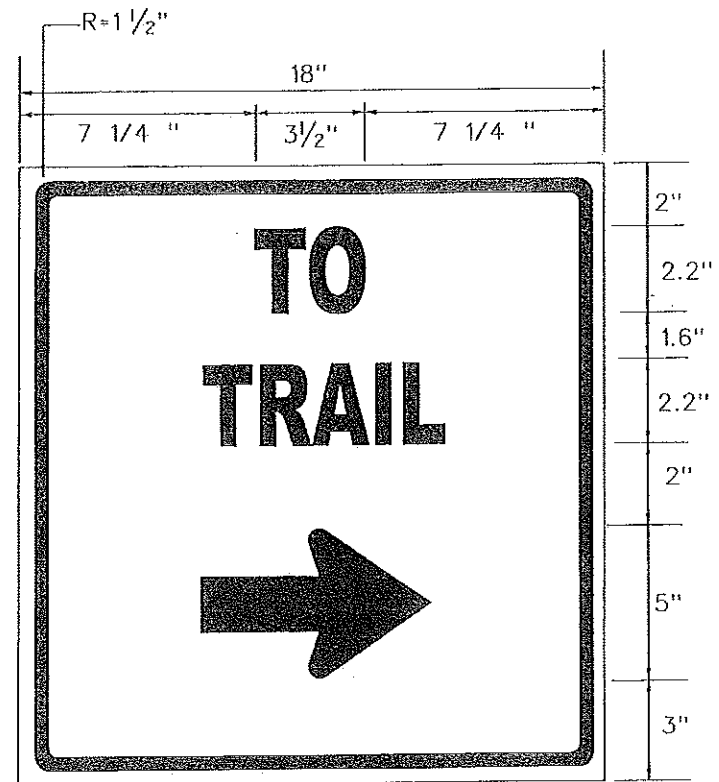
SPECIAL SIGN (18"x18") LEGEND- BLACK BACKGROUND- WHITE (REFL.) ARROW FILL WITH BLACK 2.2" LETTERS FILL W/BLACK (center of sign)
