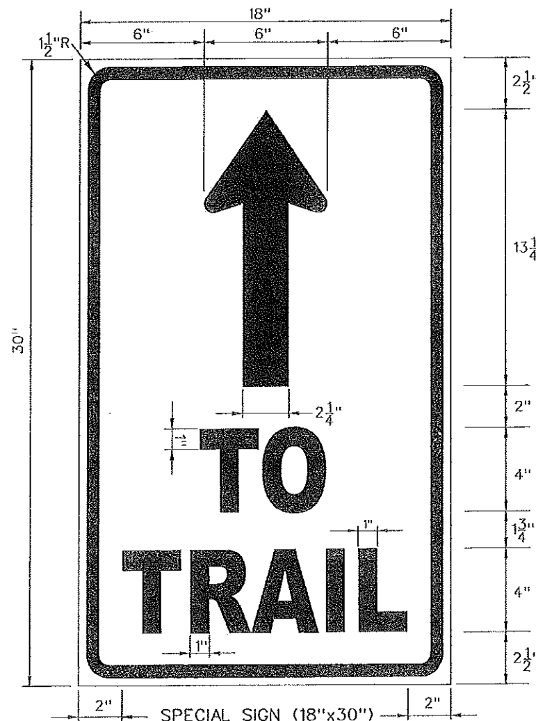
SPECIAL SIGN (18"x30") LEGEND- BLACK BACKGROUND- WHITE (REFL.) ARROW FILL WITH BLACK
