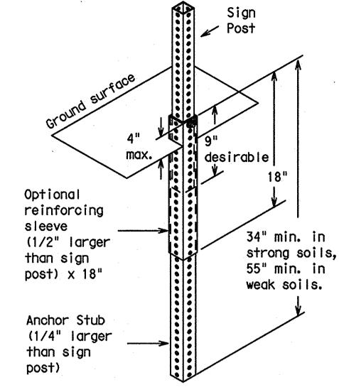
OPTION 3 (Anchor Stub and Reinforcing Sleeve))
