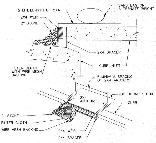
CURB INLET PROTECTION DETAIL NOT TO SCALE
