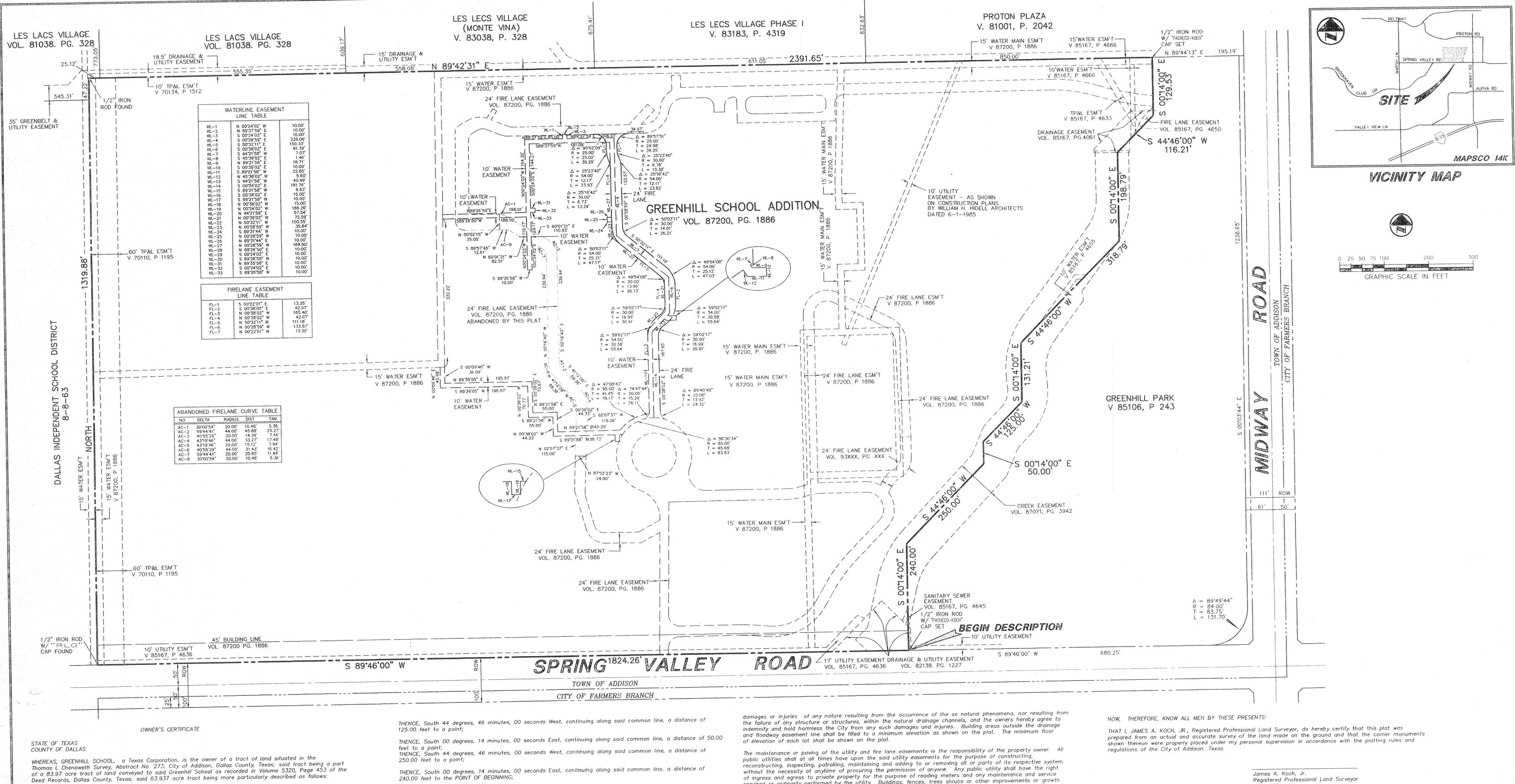
BEGINNING, at a 1/2-inch iron rod with "Pacheco Koch" cap set for corner in the north right-of-way line of Spring Valley Road (100 foot right-of-way); said point also being the most southwesterly corner of the Greenhill Park, an addition to the City of Addison as recorded in Volume 85106, Page 0243 of the Deed Records of Dallas
