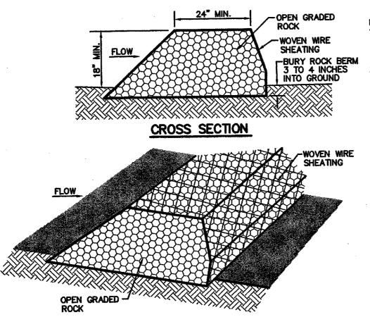
1. USE ONLY OPEN GRADED ROCK 4-8 INCHES IN DIAMETER FOR STREAM FLOW CONDITION. USE OPEN GRADED ROCK 3-5 INCHES IN DIAMETER FOR OTHER CONDITIONS. WOVEN WIRE SHEATHING HAVING A MAX OPENING OF 1 INCH AND A MIN. WRE SIZE OF 20 GAUGE AND SHALL BE BURIED IN A
