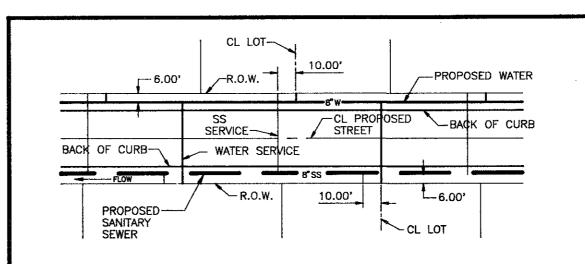
TYPICAL INSTALLATION DETAIL FOR WATER & SANITARY SEWER SERVICES **AS BUILT**
