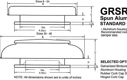
GRSR Spun Aluminum Gravity Relief STANDARD CONSTRUCTION FEATURES Aluminum housing.
