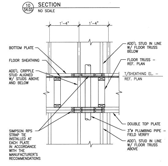
TYPICAL PLATE REPAIR DETAIL
