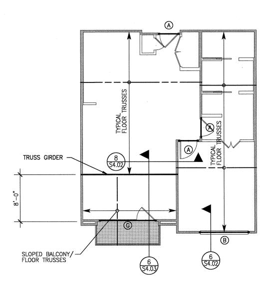
UNIT A4 1 FLOOR FRAMING PLAN \$2.03 SCALE: 1/8"=1'-0"
