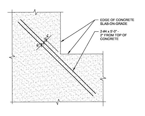
**TYPICAL RE-ENTRANT SLAB CORNER REINFORCING DETAIL** NO SCALE
