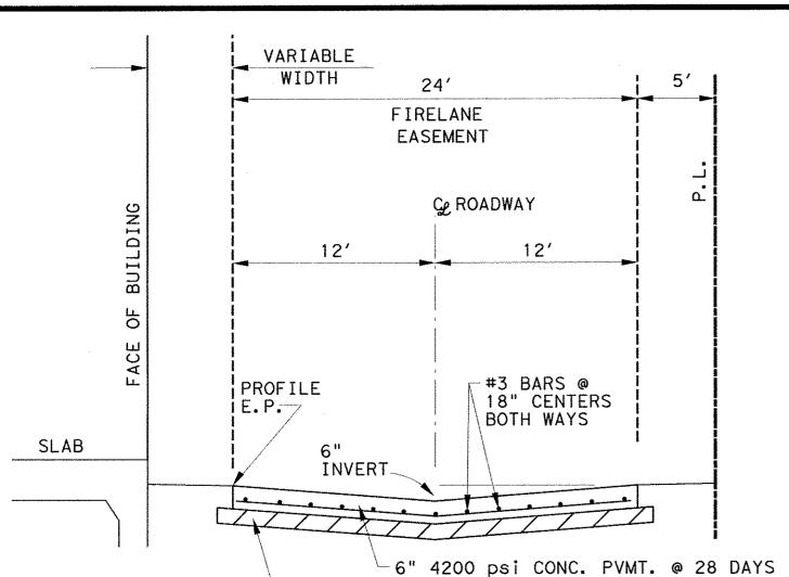
6" THICK LIME STABILIZED SUBGRADE (28 lbs/sy) -COMPACTED TO A MIN. 95% OF STANDARD PROCTOR DENSITY @ 0% TO +3% OF OPTIMUM MOISTURE
