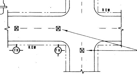
A BLUE STIMSONITE FIRE-LITE REFLECTOR (OR APPROVED EQUAL) TO BE PLACED IN THE CENTER OF STREET DPPOSITE FIRE HYDRANTS. THE INSTALLATION OF THIS REFLECTOR SHALL BE AS PRESCRIBED BY THE MANUFACTURER.
