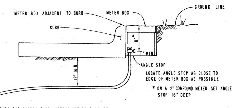
" MIN. TYPE "K" COPPER (ASTM SPECIFICATION B 88-55 AND AWWA SPECIFICATION 75-CR)
