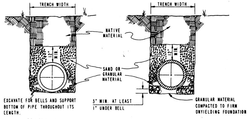
( C.I. OR D.I. PIPE ) TYPICAL BACKFILL (C.I. OR D. I. PIPE) WATER MAIN
