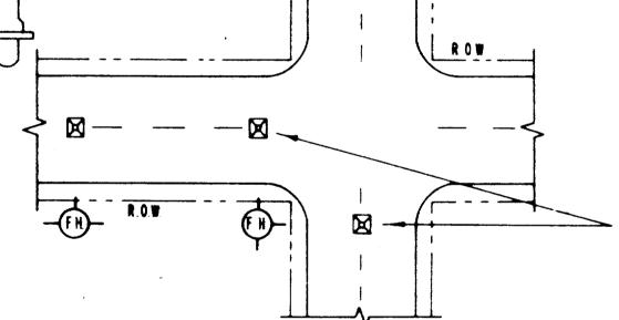
A BLUE STIMSONITE FIRE-LITE REFLECTOR (OR APPROVED EQUAL) TO BE PLACED IN THE CENTER OF STREET OPPOSITE FIRE HYDRANTS. THE INSTALLATION OF THIS REFLECTOR SHALL BE AS PRESCRIBED BY THE MANUFACTURER
