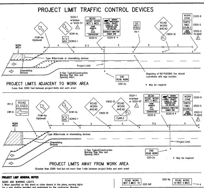
1. When specified on this sheet or other sheets in the plans, warning lights for a sign shall be installed and maintained by the contractor. Warning lights shall be attached to the sign support using a 1/2" bolt (minimum) of sufficient length for three washers, lock washer and a nut.
