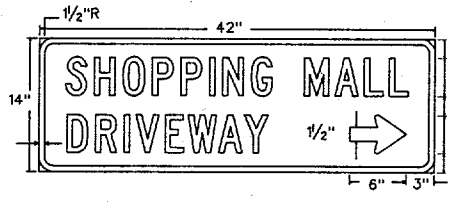
D-70S 42" X 14" Letters - White Refl. Symbol - White Refl. Border - White Refl. Background - Blue Refl.
