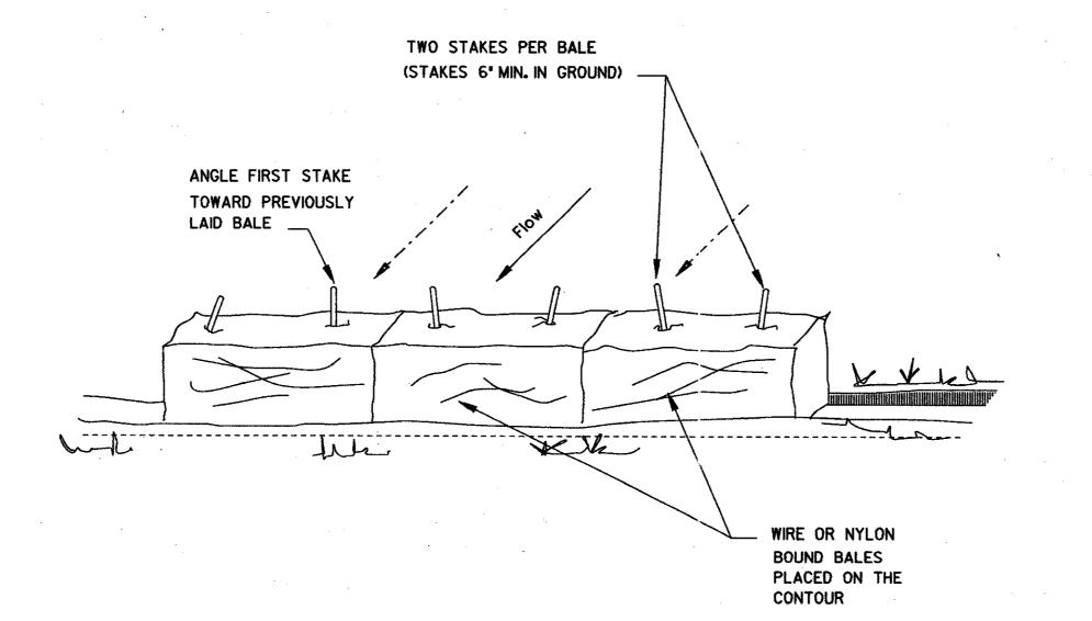
ANCHORING DETAIL FOR HAY BALE DIKE
