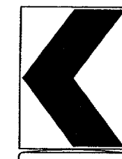
18" x 24" Sign (Maximum Sign Dimension) Chevron CWI-8, Driveway sign D70a, Keep Right R4 series or other signs as approved by Engineer
