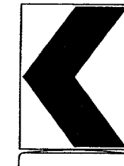
18' x 24' Sign (Maximum Sign Dimension) Chevron CWI-8, Driveway sign D70a, Keep Right R4 series or other signs as approved by Engineer
