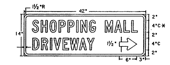
D-70S 42" X 14" Letters - White Refl. Symbol - White Refl. Border - White Refl. Background - Blue Refl.
