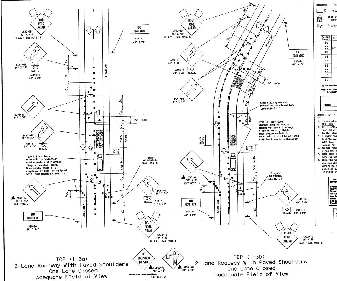
LEGEND \_ ■ Channelizing Devices Type III Barricade Heavy Work Vehicle Truck Mounted Attenuator Portable Changeable Flashing Arrow Panel Message Sign ≖a Sign Post
