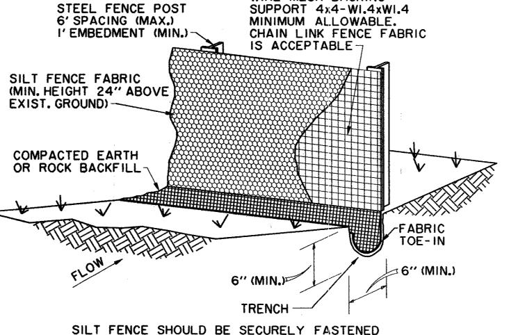
SILT FENCE SHOULD BE SECURELY FASTENED TO BACKING SUPPORT AND POSTS.
