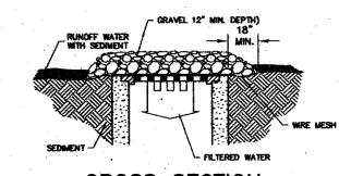
THIS METHOD OF INLET PROTECTION IS APPLICABLE WHERE HEAVY CONCENTRATION FLOWS ARE EXPECTED, BUT NOT WHERE PONDING AROUND THE STRUCTURE MIGHT CAUSE EXCESSIVE AND UNPROTECTED AREAS
