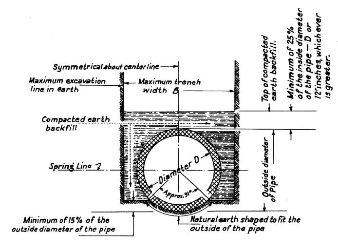
TRENCH BEDDING IN EARTH FOR PRECAST PIPE WITHOUT CONCRETE CRADLE OR CUSHION
